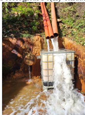
Fig. 1. Mine water discharge from the flooded Manó–Gabriela siderite mine at the Marta adit, Nižná Slaná, Slovakia.
