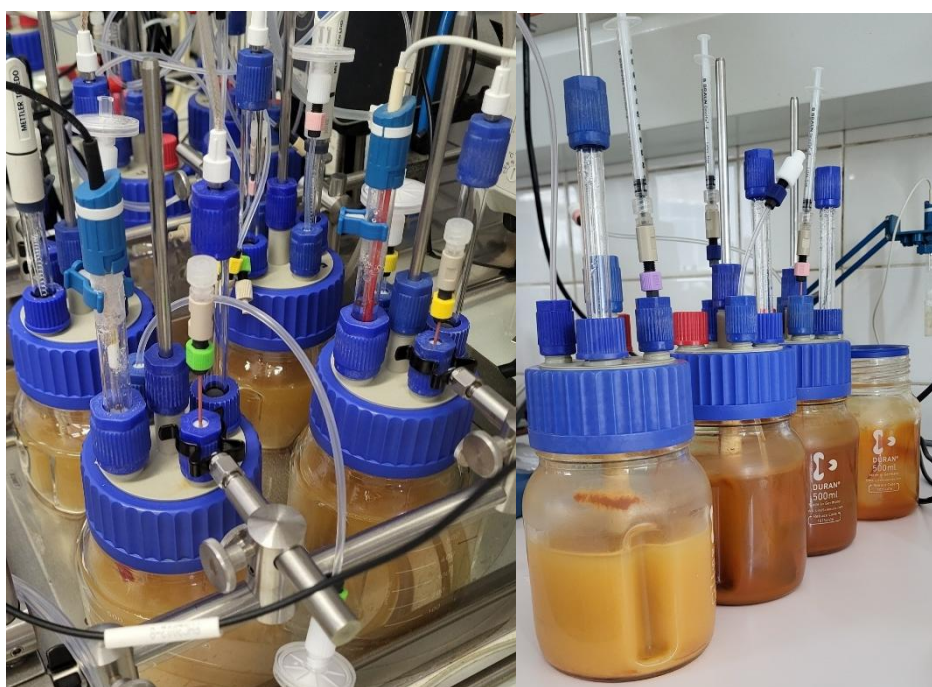
Fig. 1. Experiment set-up consisting of four 0.5 L reactors connected to online gas analysis, operated under stable temperature conditions, followed by pH adjustment and subsequent equilibration.
