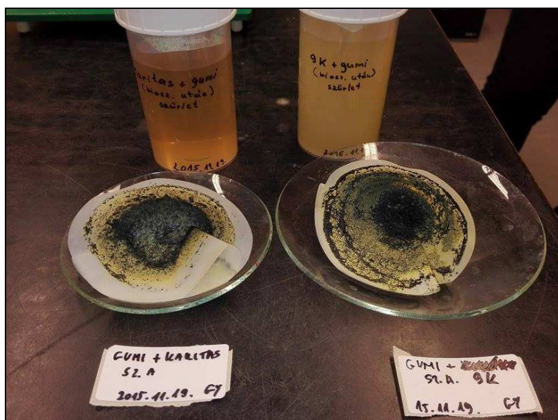
Fig. 4. Solid and liquid phases after the bioleaching with Acidithiobacillus ferrooxidans Karitas (left) and leaching with 9K (right)
