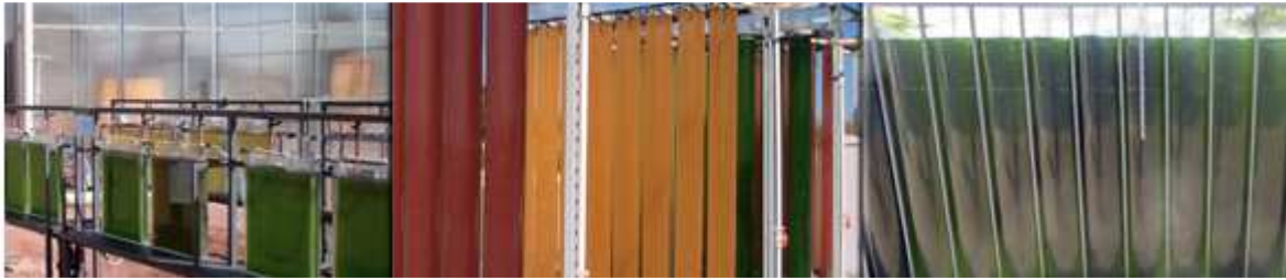
Fig. 5. Closed systems for algae cultivation: flat-plate, horizontal tubular and polybags [10]
