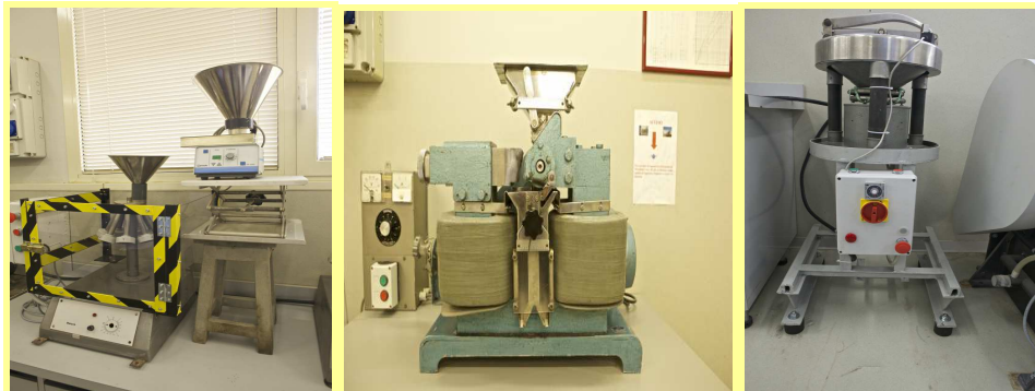
Fig. 2. Equipment used for physical treatment (sampling, magnetic separation, milling)
