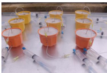
Fig. 1 The stabilization of contaminated soils using nZVI (batch experiment)
